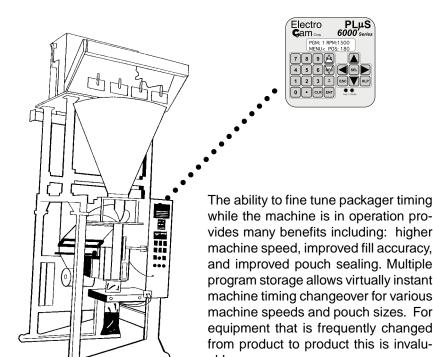
Speed compensation automatically advances and retards the output setpoints as the machine speeds up and slows down. This feature is particularly valuable when controlling slow moving mechanical devices. When speed compensation is used, changes in production speed do not require setpoint changes. Outputs are properly synchronized while ramping up to speed or slowing down to a stop.
